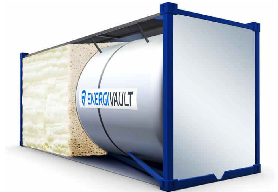
Figure 21 - example of a latent heat CTES storage tank. This particular implementation uses water-ice as the phase change material; this is what is stored in this tank. See the later case study for further details. Source: Organic Heat Exchangers Ltd.
