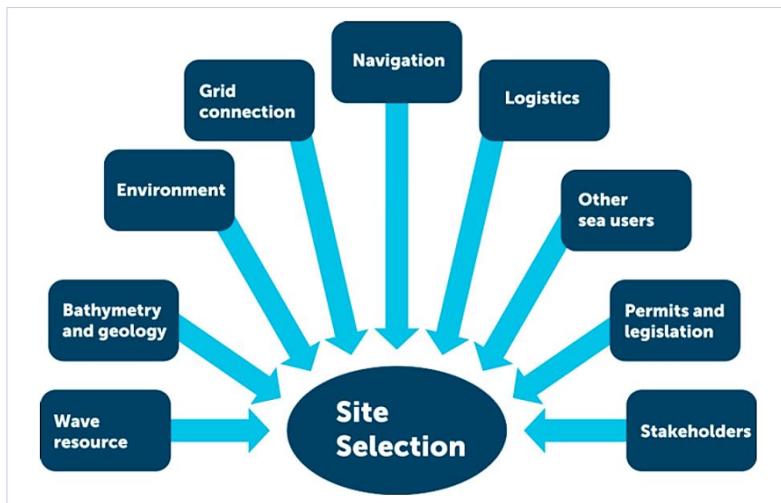
Figure 2 - factors that go into site selection for an OE project (example uses wave energy specifically). Bathymetry is the study of underwater depth. Geology is important for some devices fixed or moored to the ocean bed.
