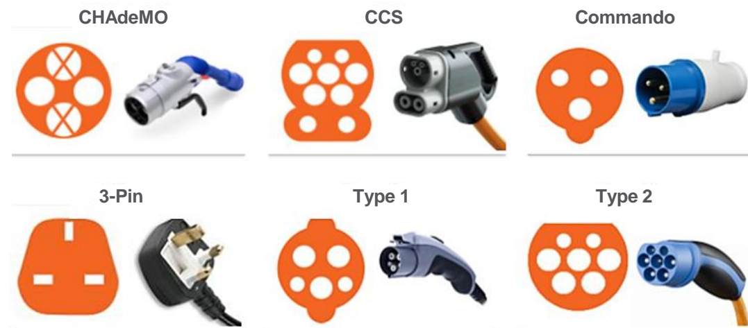
Figure 16 - the main types of EV charging cable connectors. Rapid chargers use CHAdeMO, CCS or Type 2 connectors. Fast and slow chargers use Type 2, Type 1, Commando, or 3-pin plug outlets. Image source .
