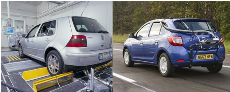
Figure 12 - lab-based rolling-road testing, left, versus Real Driving Emissions (RDE) testing, right. Image source: Next Green Car .
