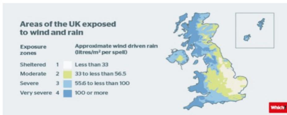
Figure 3 - Areas of the UK exposed to wind and rain <sup>9</sup>. Houses in the areas marked 'very severe' may potentially develop problems with existing CWI, or may not be suitable for new CWI.
